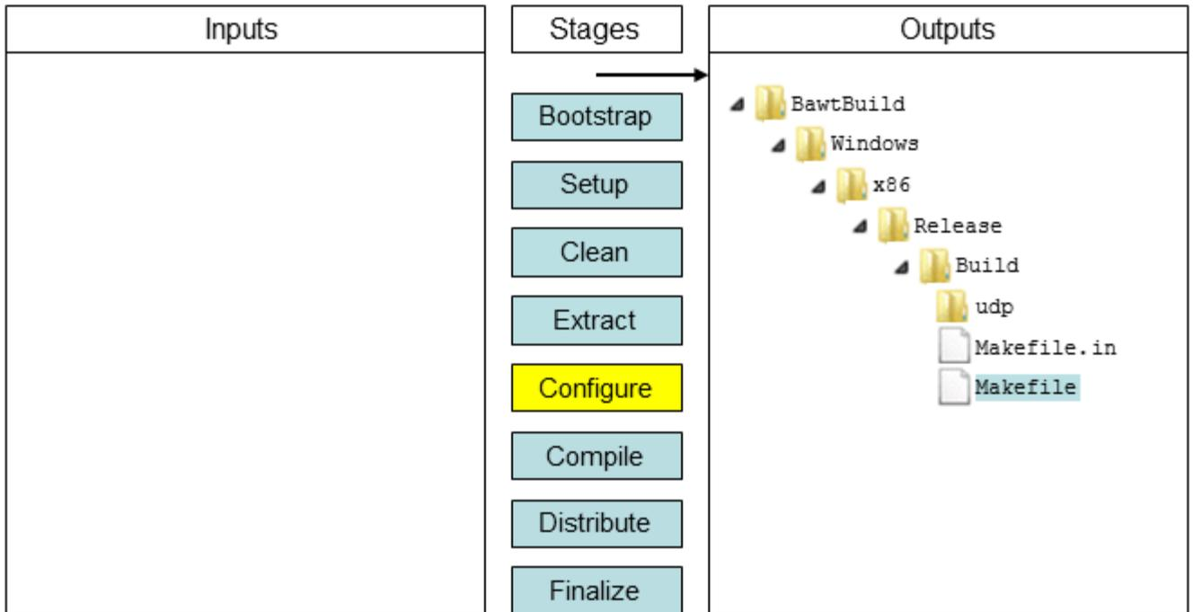
In stage `Configure` the library will be configured, which generates the appropriate make files for the chosen compiler and platform.
