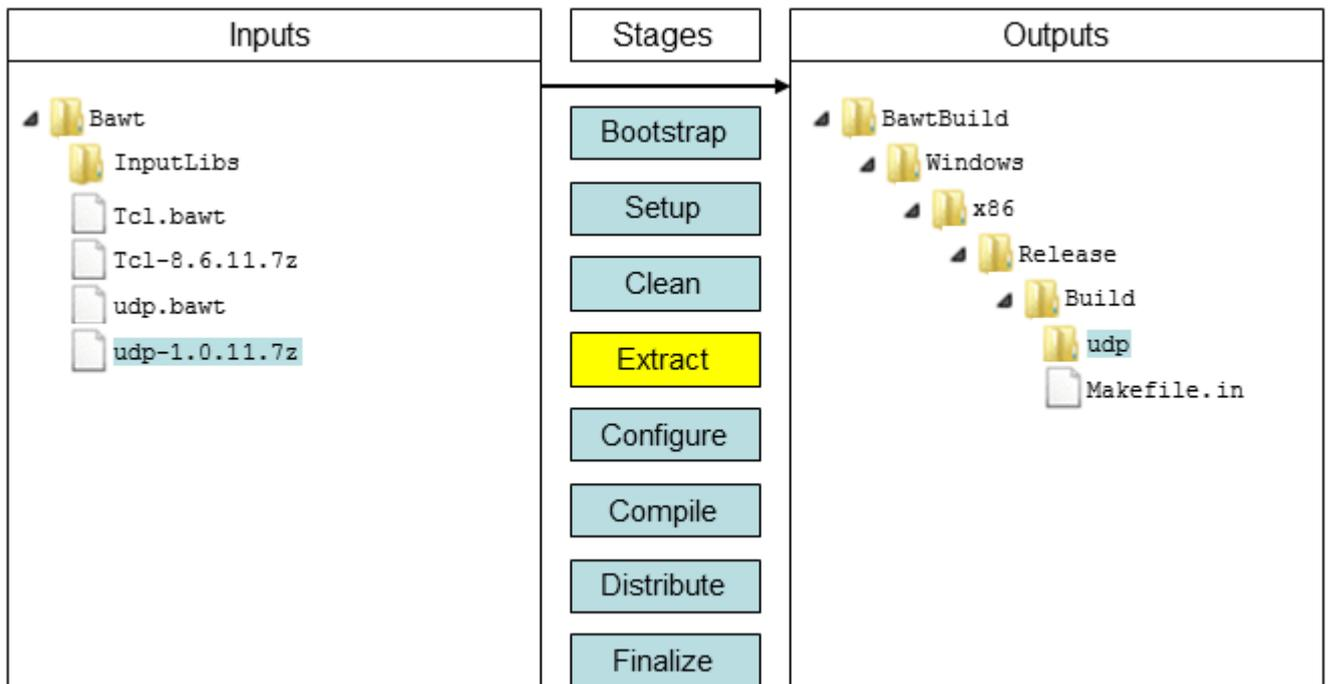
In stage `Extract` the library source code will be extracted and copied into the build directory. This is achieved by calling the **BAWT** procedure `ExtractLibrary`, which cares about having either a source directory or a compressed source file.
